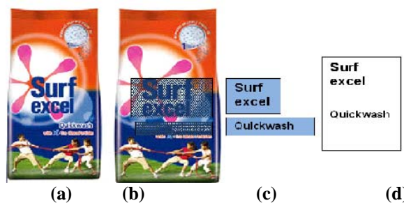
Fig.2. Example of text localization and recognition from camera captured images. (a) camera captured images. (b) Localized text regions (marked in blue). (c) Text regions cropped from image. (d) Text codes recognized by OCR.
